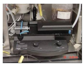
Picture 4: Syringe pump, Sage Model M365
