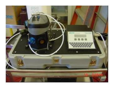
Picture 2: Leak detector Model TDA-99M
