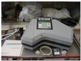
Picture 9: Miran Analyzer, Model 1A
