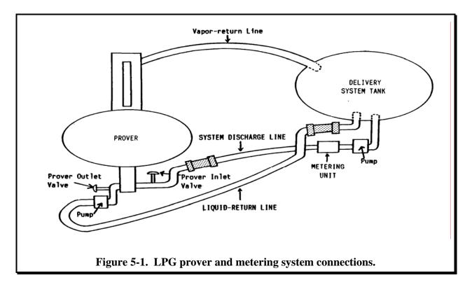
Because the product must be maintained in its liquid state for accurate measurement, the prover is closed and pressure-tight and is connected in such a way as to become incorporated with the
