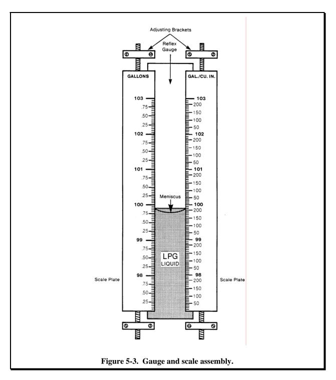
You should be at eye level with the liquid level in the gauge when reading the gauge. The top surface of the liquid may be slightly concave, and so when viewed from this position may appear to have two surfaces, one flat and a lower one that is slightly curved. This curvature results from capillary attraction of liquid to the gauge glass. The apparent curved level when viewed from the side is called the <u>meniscus</u>.
