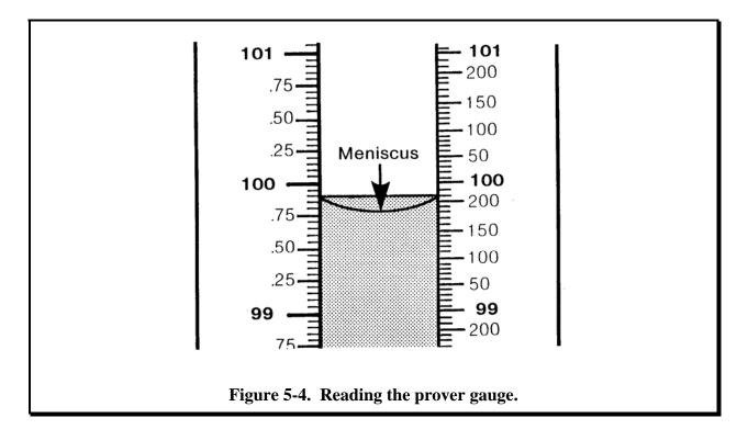
For example, the bottom of the meniscus shown in Figure 5-4 appears to coincide with a point exactly midway between the graduations that represent 99.75 and 99.80 gal on the left-hand scale, and coincides most closely with the graduation representing 99 gal plus 180 cu in on the right-hand scale. In this case, the reading should be recorded either as 99.80 gal or as 99 gal plus 180 cu in.
