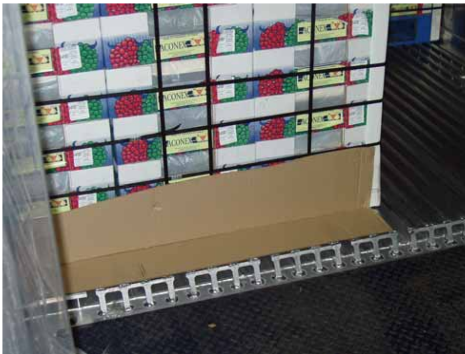
FIGURE 3-7-5 Proper placement of cardboard between the last pallet row of fruit and the back doors of the container
