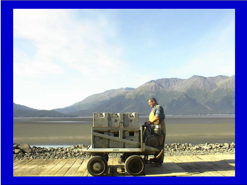
Test cart with two tiers of weights properly stacked inside. Notice how weights are balanced between the wheelbase of the cart.
