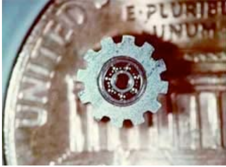
LIGA-micromachined gear for a miniature electromagnetic motor.
