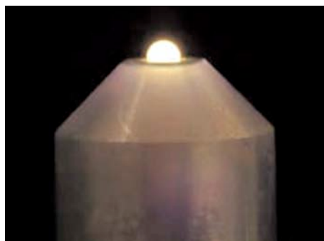
Levitated liquid aluminum oxide sample in a super-cooled state at ~1800° C.
