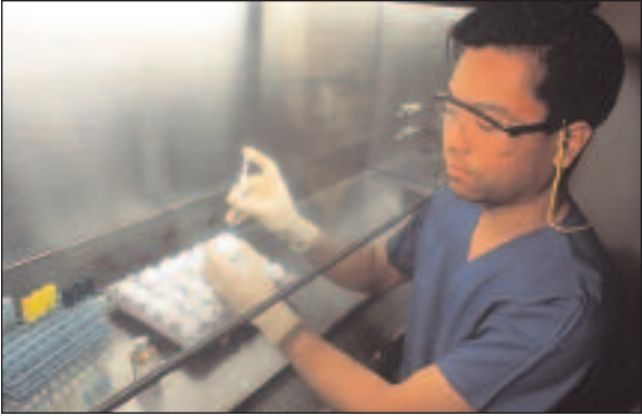
Figure 1 —A microbiologist inoculates eggs free of specific diseases to determine the viral titer of a poultry vaccine.
