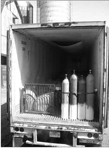
Figure 12.1. A reefer style semi-trailer has been modified to dispense CO 2 gas to euthanize swine during a depopulation of a PRV-infected herd. (APHIS photo by Doris Olander)
