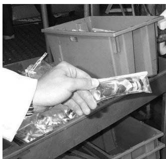
Figure 8.5. Meat sample sealed in a container and identified by sample number. Will be frozen overnight then thawed to yield meat juice for testing. (APHIS photo by Lowell Anderson)
