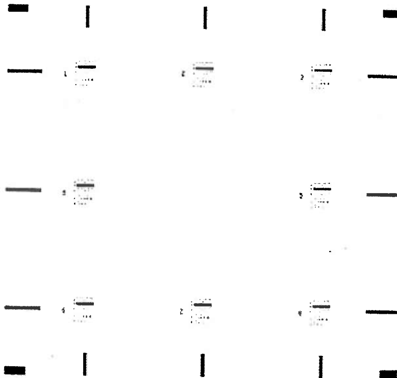
Figure 2. A view of the center of SRM 476. The pattern number given with the serial number identifies which pattern has been certified by NIST. Pattern identification numbers can be seen to the left of each basic measurement pattern.
