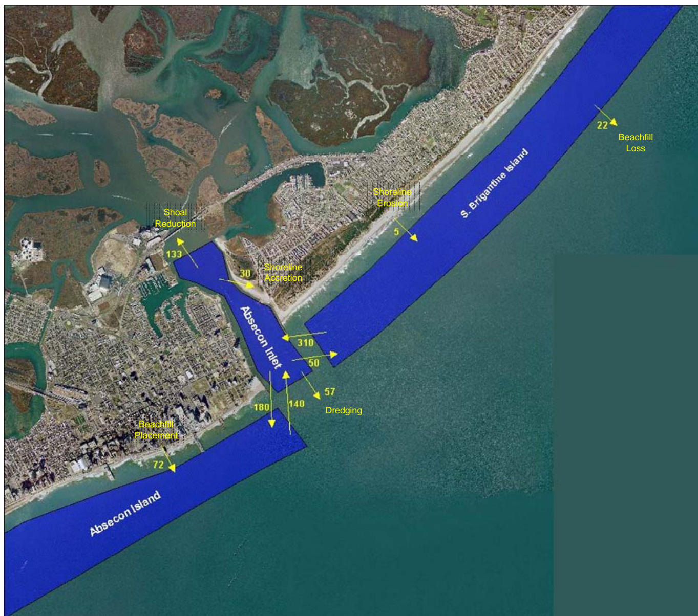
Figure 8. Sediment Budget for Absecon Inlet and Vicinity (1000x yds 3 / yr)
