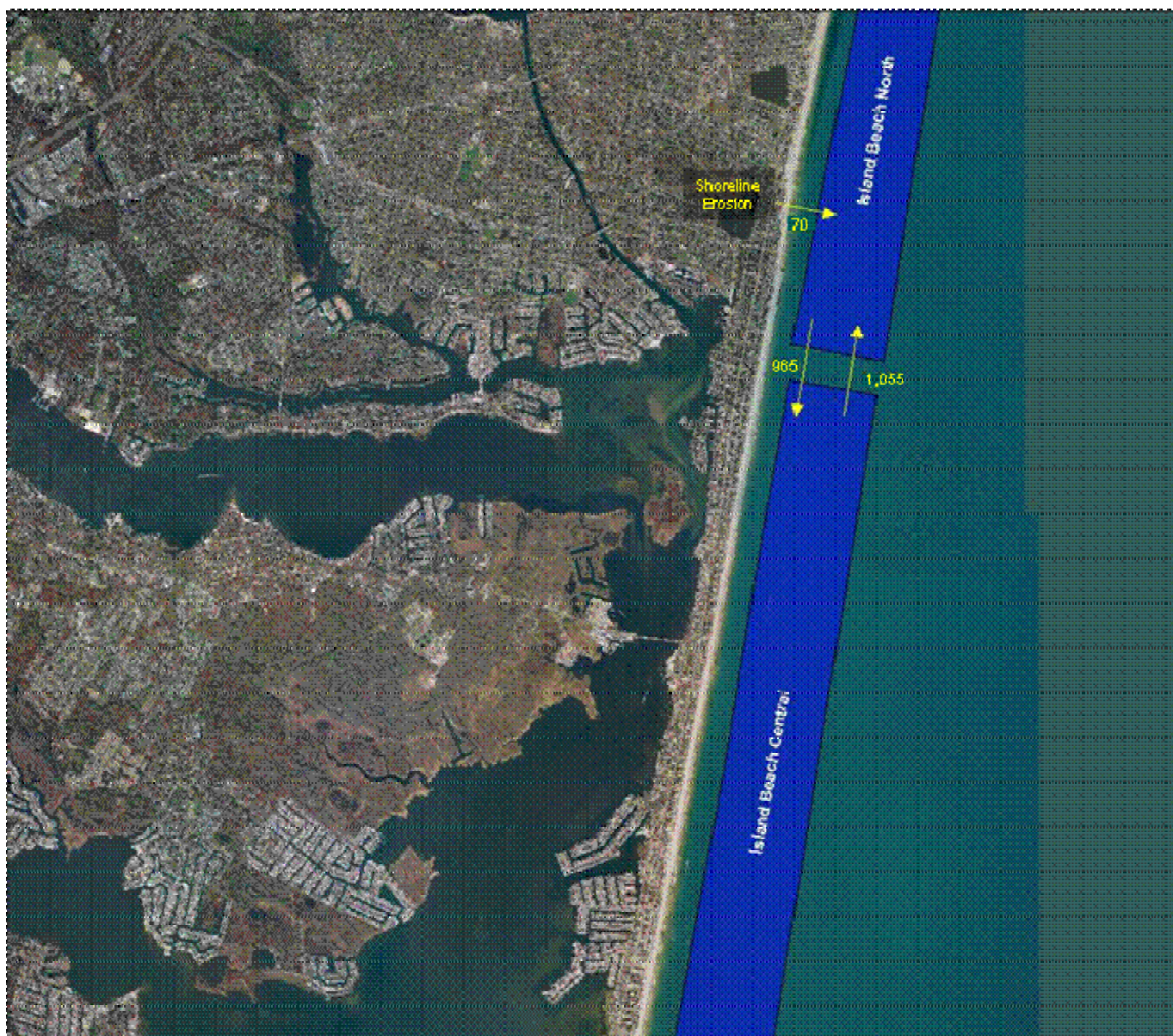
Figure 17. Sediment Budget for North Island Beach ( 1000x \text{ yds}^3 / \text{yr} )
