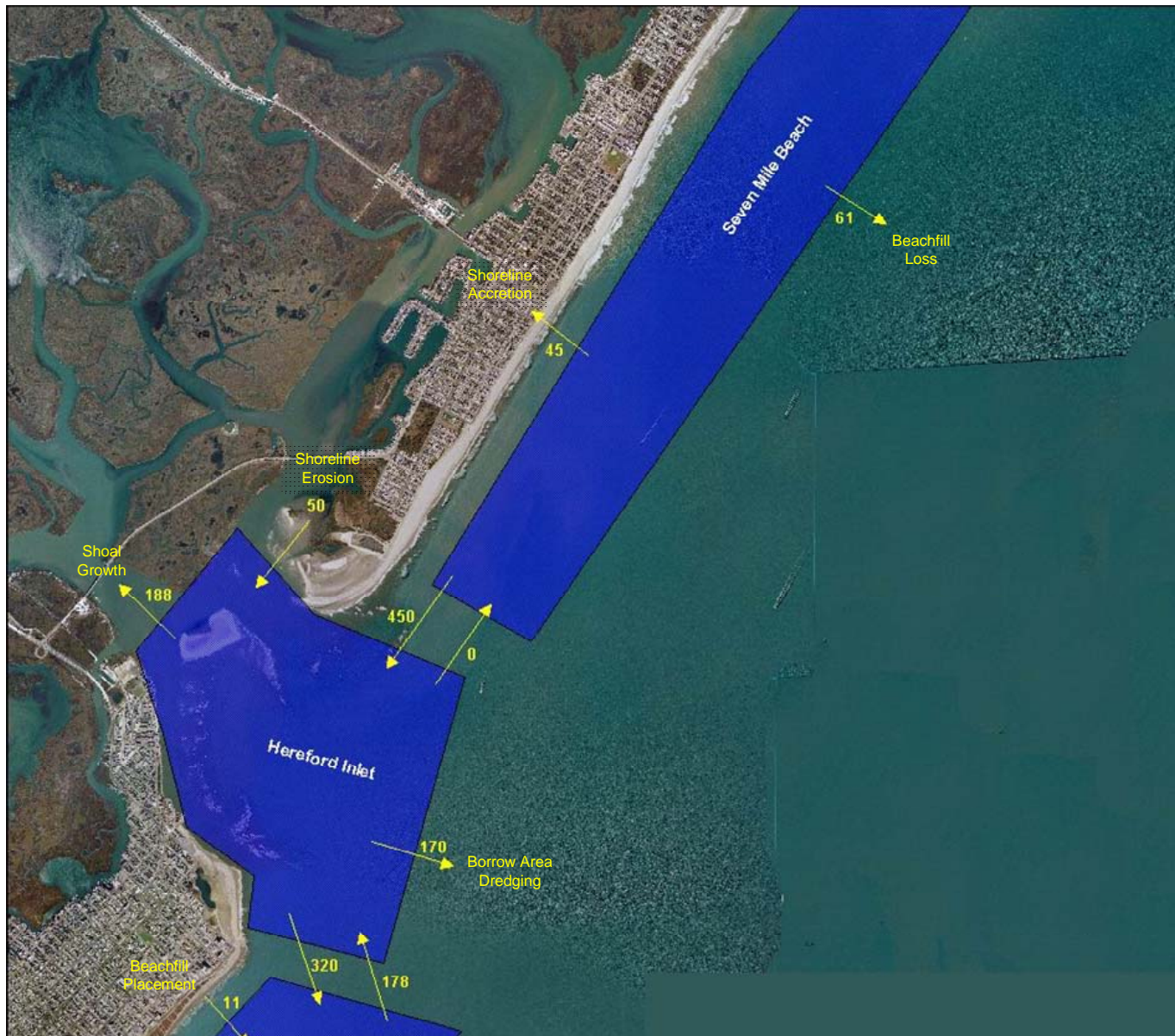
Figure 3. Sediment Budget for Hereford Inlet and Vicinity (1000x yds 3 / yr)
