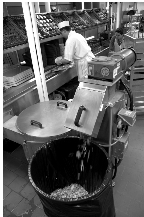
(from left) Food service workers Alekos Polyzos and Crystal Cavin break down breakfast trays for the dish room pulper. The team dumps food and paper items into the water flowing over the conveyor belt, which moves it forward, and stacks the dishes into a machine that washes, rinses, dries them. The pulper gurgles and thumps as it extracts the liquid from the items and chops them into tiny pieces.
