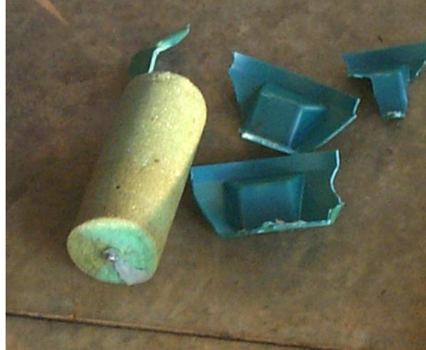
Figure 1-2. Shattered Dewar plug
