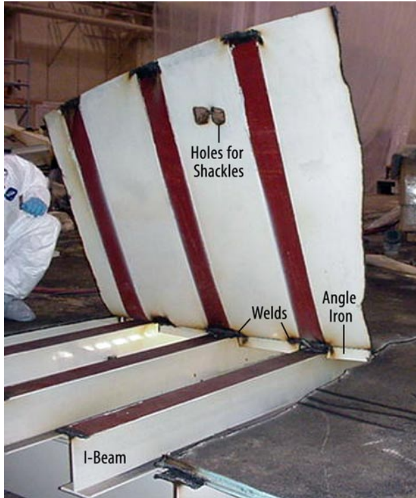
Figure 2-1. Steel plate section of tank floor
