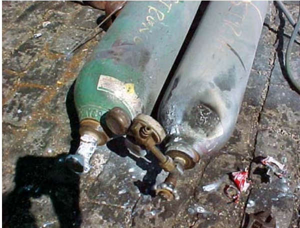
Figure 4-2. Oxygen cylinder burned during fire
