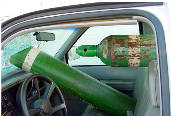
Figure 4-1. Unsecured cylinders during transport
