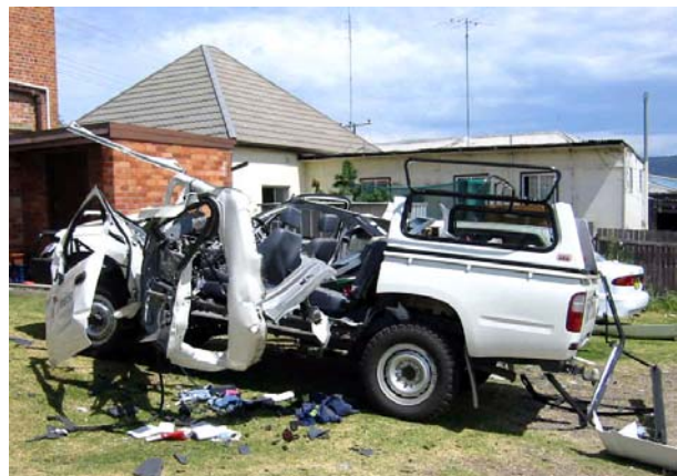
Figure 4-3. Acetylene cylinder explosion
