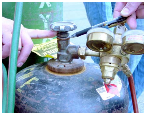
Figure 4-1. Fire originated between the isolation valve and packing nut
