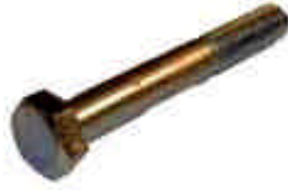
Figure 2-1. Grade 2 bolt with no manufacturer's headmark
