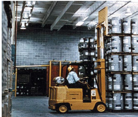
Figure 2-1. Typical propane-powered forklift operating indoors
