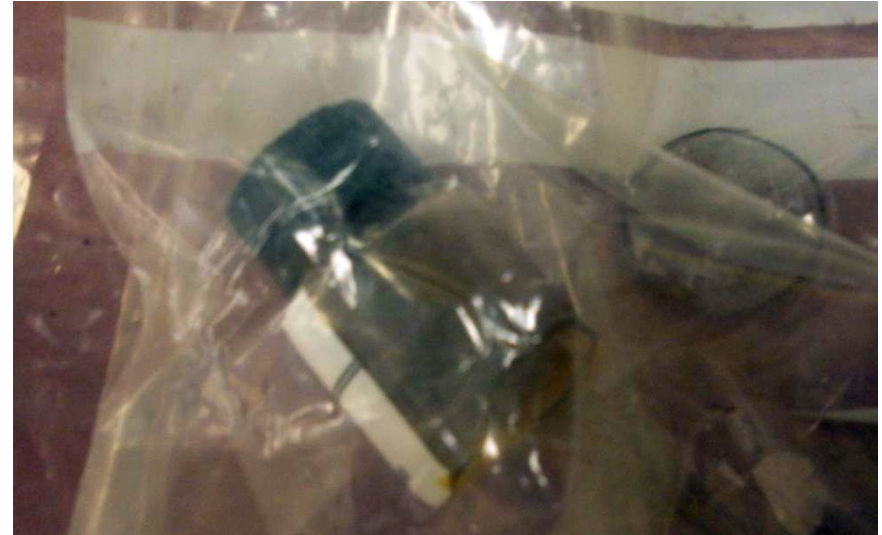
Figure 1-1. Broken glass container inside multiple plastic bags (broken bottom in upper right-hand corner)
