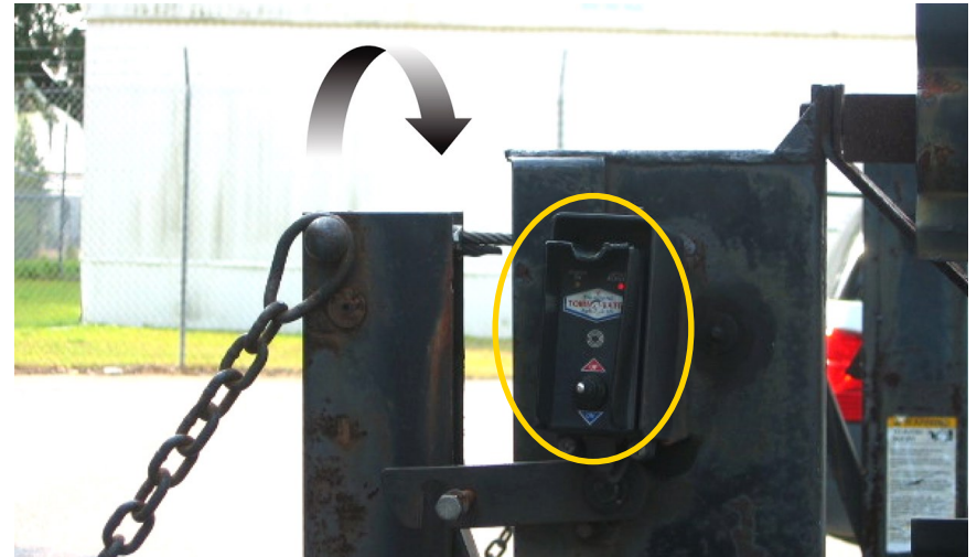
Figure 2-1. Control switch (circled) on right side of the delivery truck (arrow shows the scissor-like movement of the mechanism)
