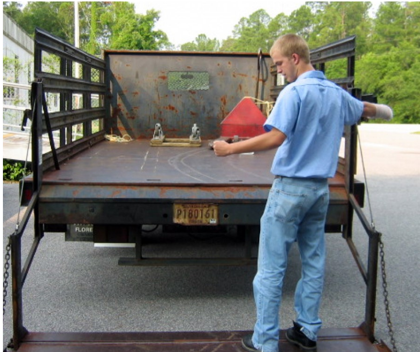
Figure 2-2. Injured worker reenacts the accident, showing how he was positioned on the lift while operating the control switch (note worker's bandaged arm)
