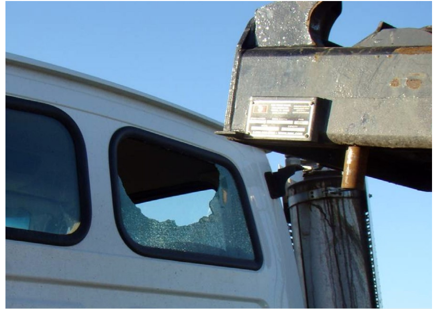
Figure 1-1. Passenger side rear window damage
