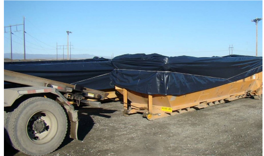
Figure 1-2. Empty container after sliding off rails
