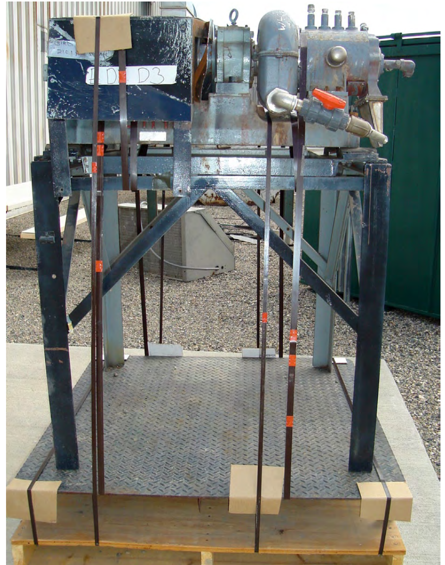
Figure 2-1. The pump assembly shown banded back together on the metal skid after the incident
