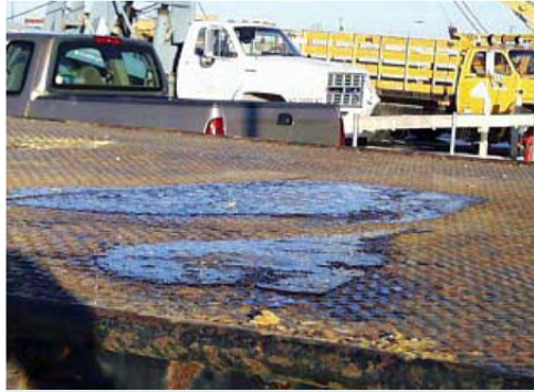
Figure 2-4. Ice on metal bed of trailer
