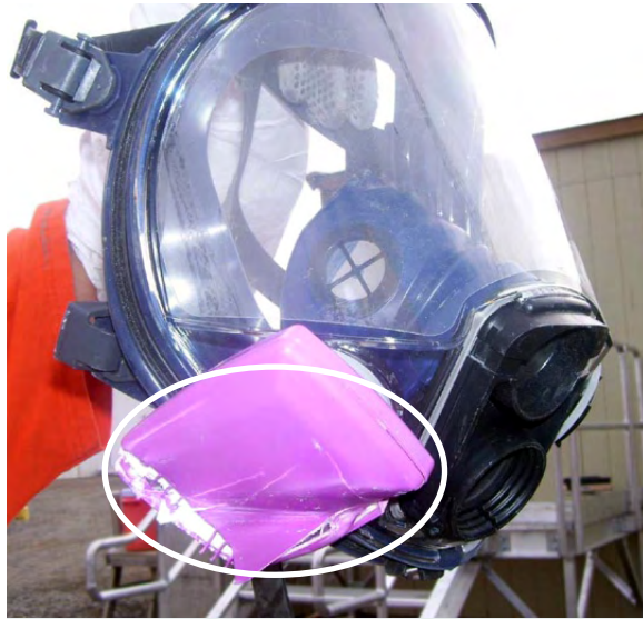
Figure 1-2. Damage to pink filter on painter's respirator
