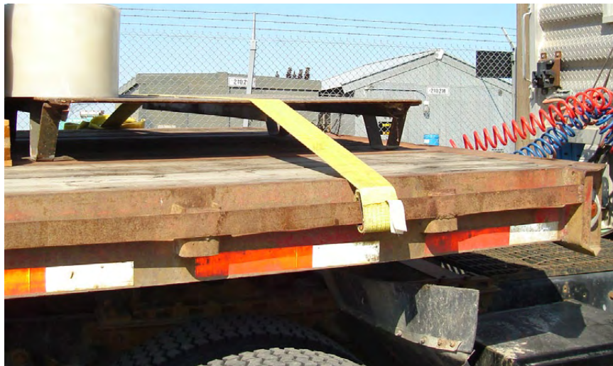
Figure 2-3. Metal skid held down by yellow strap
