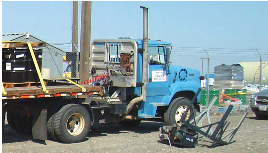
Figure 2-2. Tractor-trailer and fallen pump assembly
