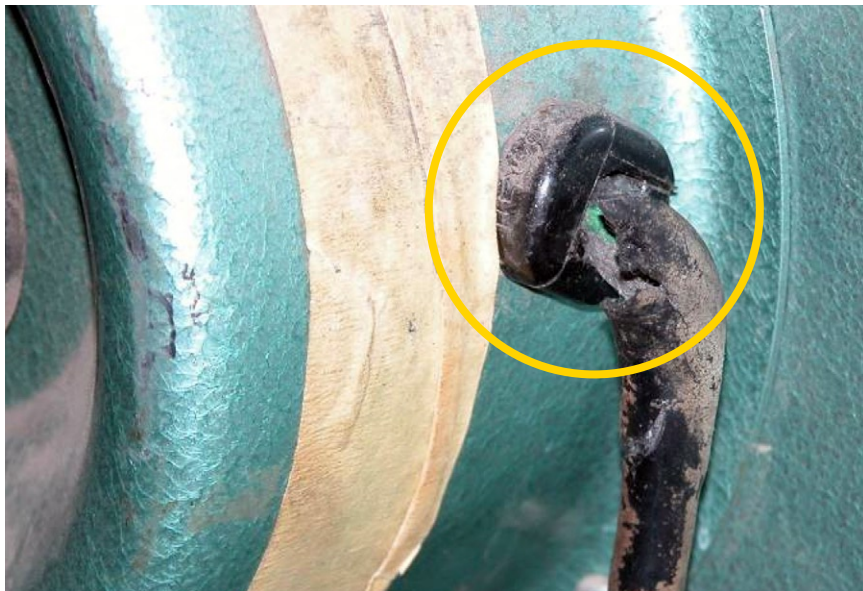
Figure 1-2. Damaged power cord
