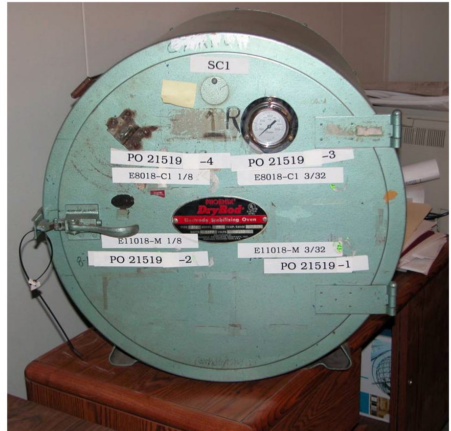
Figure 1-1. Welding rod oven
