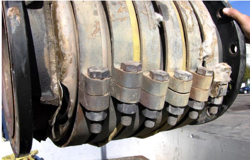
Figure 1-2. Ruptured expansion joint shown after removal
