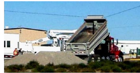
Figure 3-1. Truck bed caught on power line
