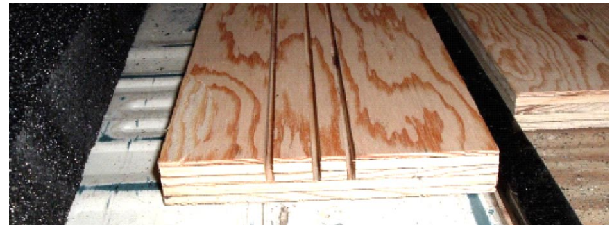
Figure 1-2. Dado cuts in plywood
