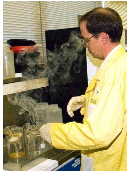
Figure 3-1. Re-enactment of event showing how vapor passed through workers' breathing zone
