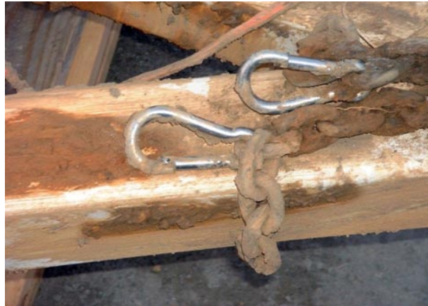
Figure 3-3. Post-accident photo showing unattached safety chains
