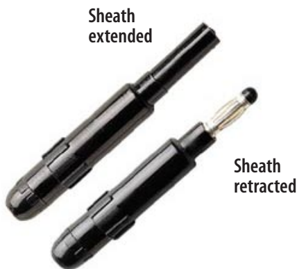
Figure 2-4. Typical retractable-sheath banana plug
