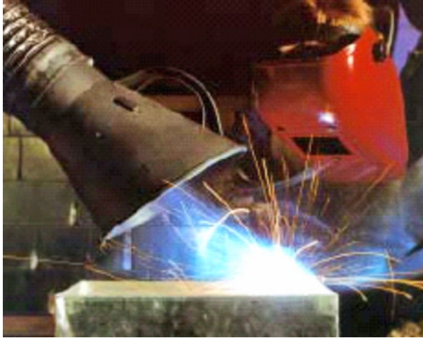
Figure 1-1. Using local exhaust ventilation at the work piece
