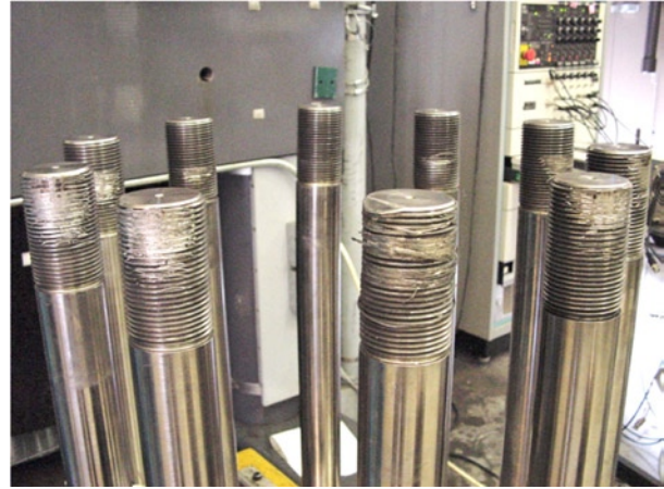
Figure 3-3. Stripped threads on tie rod ends
