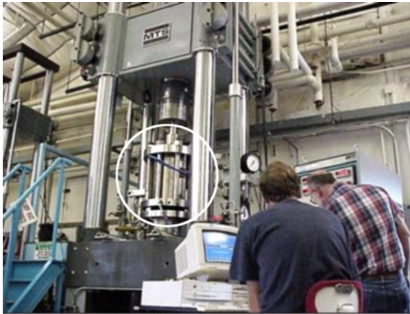
Figure 3-2. Assembled pressure vessel (circled) in the loading frame
