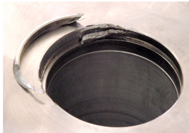
Figure 3-4. Metal fragment from o-ring groove
