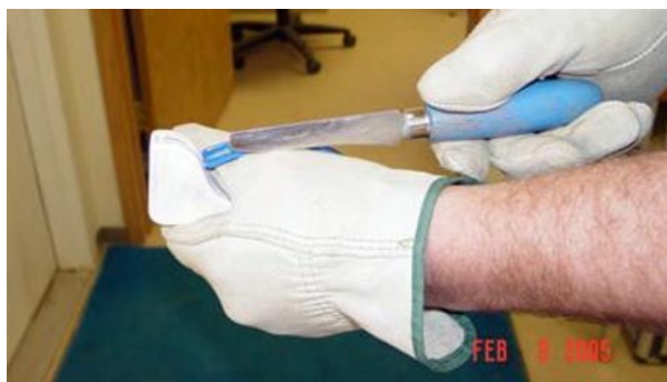
Figure 1-2. How the worker used the sharpener
