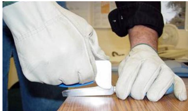
Figure 1-3. Correct use of the knife sharpener
