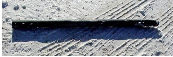
Figure 2-2. Piece of conduit used as a cheater bar
