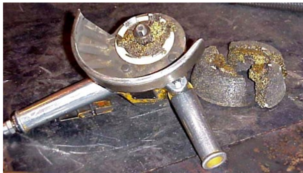
Figure 2-3. Damaged grinder and cup stone
