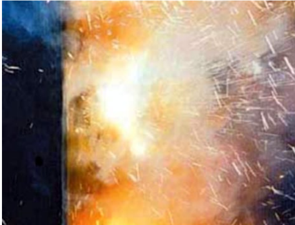
Figure 3-4. An electrical arc flash test
