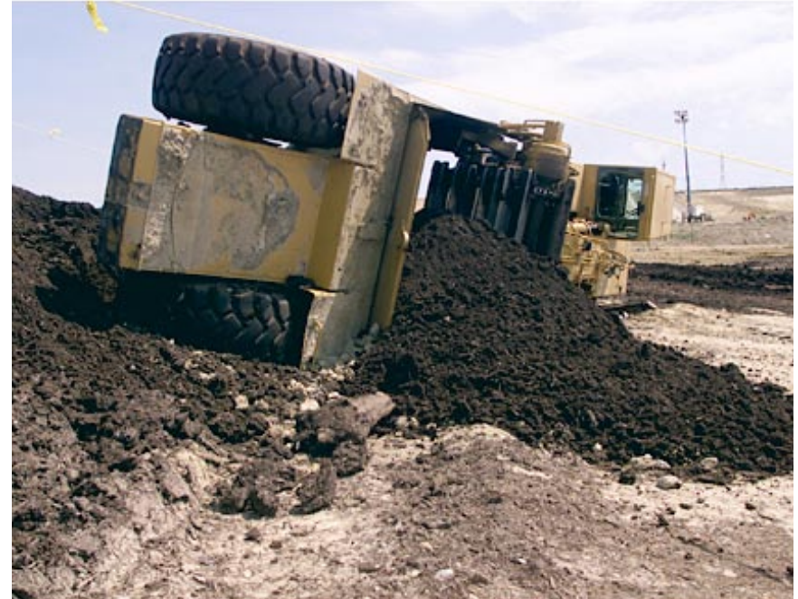
Figure 3-1. Scraper following rollover
