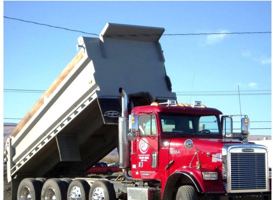
Figure 1-1. Raised bed in contact with power line
