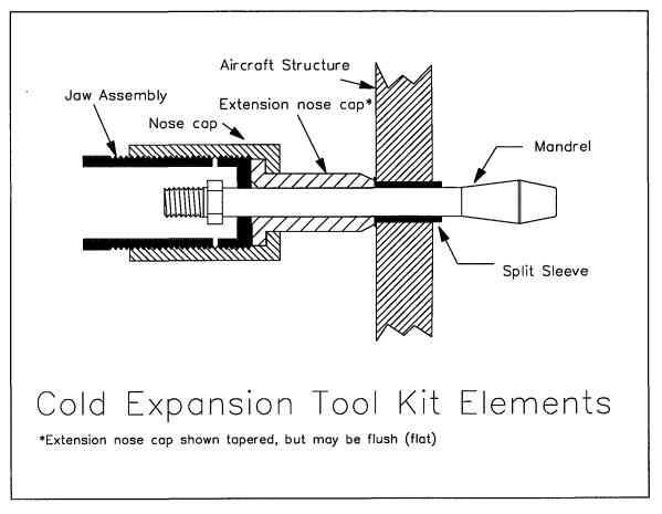
Field Tool Kits. Field tool kits consist of the same basic tools as the depot kit, however, the field tool kits are designed to cold expand fastener holes from 3/16" inch to 3/8" inch diameter.
