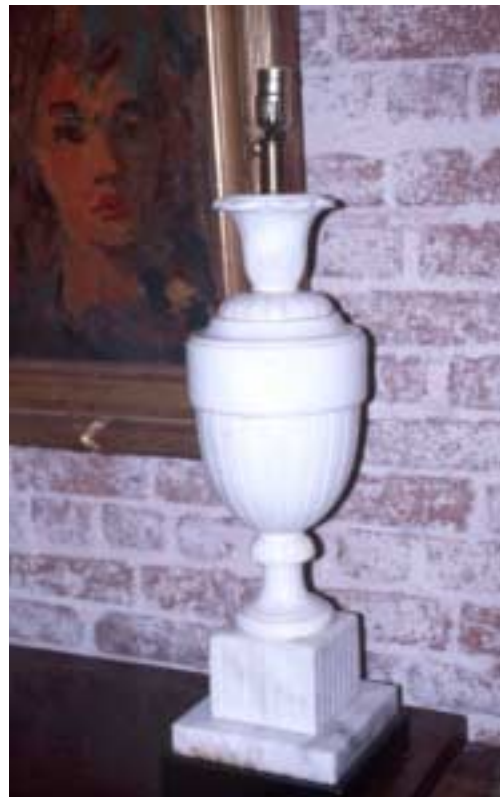
Figure 3. A lamp base comprised of five separate turned and carved alabaster components, joined with a threaded steel rod. Over-tightening can cause damage to edges of the alabaster sections.
