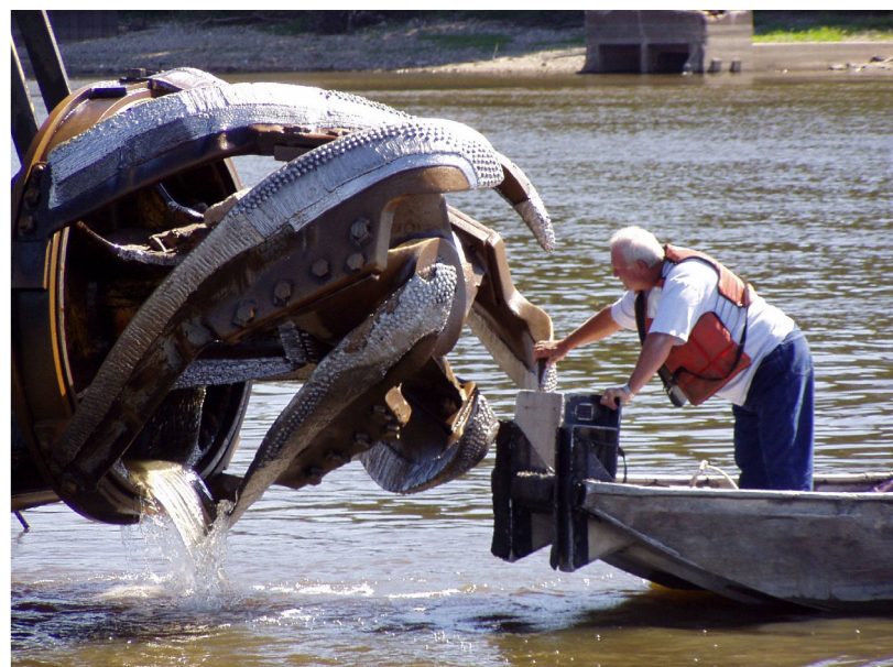
Left - Sediment is deposited on a river shoreline during dredging operations in August 2000. Above - An illustration of a typical cutterhead dredging operation used by the District. Right - One of the most important pieces of equipment in dredging, the cutterhead, is closely inspected during dredging operations.
