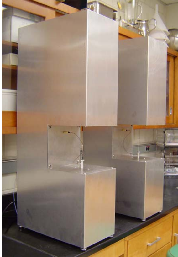
FIGURE 2. PROTOTYPE FLAMMABILITY TESTERS SHIPPED TO LICENSEES. POC: Richard E. Lyon, Ph.D., Manager Fire Research Program, Federal Aviation Administration, William J. Hughes Technical Center, Atlantic City International Airport, New Jersey 08405; Phone (609) 485-6076; Email: richard.e.lyon@faa.gov.
