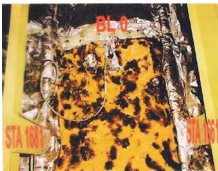
Typical PET Insulation Burn
