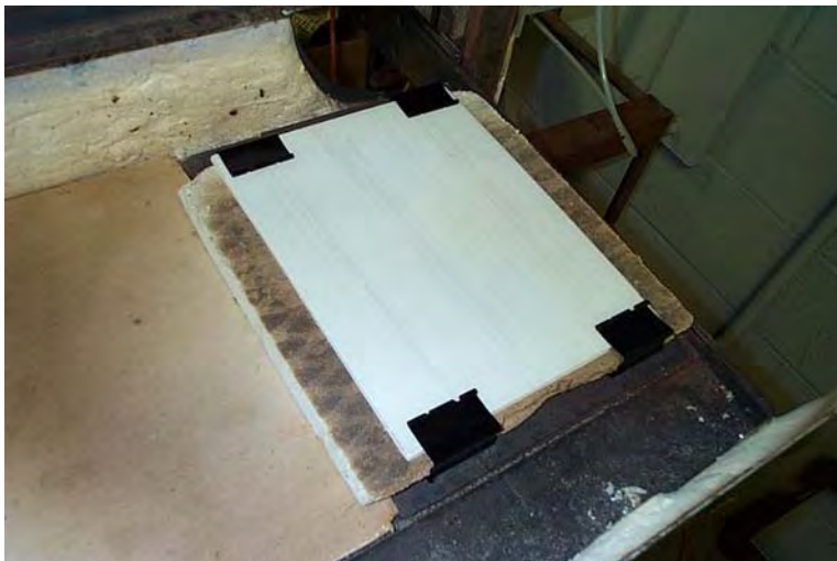
Figure 4. Example of Clamped Radiant Heat Panel Test Specimen
