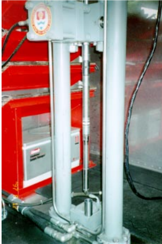
Figure 5. DL-LIBS probe including soil moisture and stratigraphy sensors, shown installed in SCAPS truck
