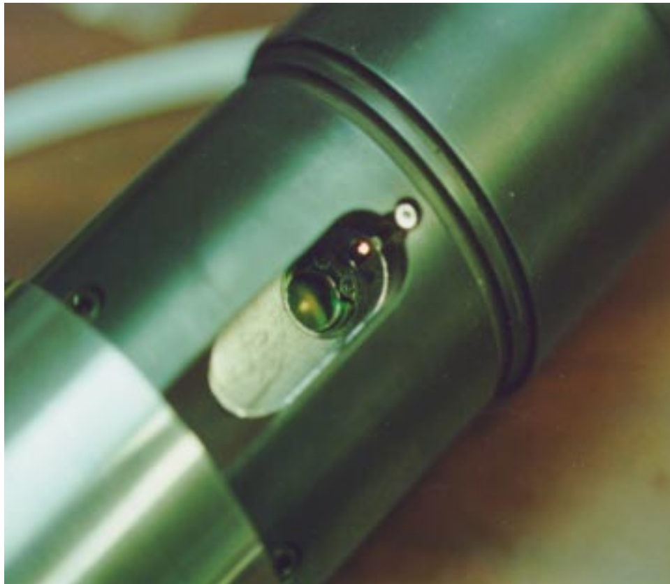
Figure 4. Closeup view of recessed window area and slot geometry of DL-LIBS probe
