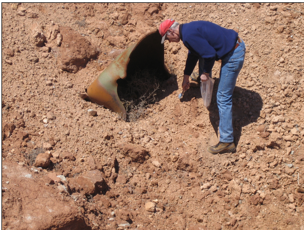
Figure 2-12. Soil sampling being conducted near a low-order 2,000-lb bomb at Holloman Air Force Base, NM.
