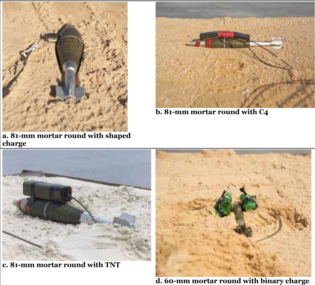
Figure 6-3. 81-mm mortar rounds with (a) shaped charge, (b) C4, and (c) TNT; (d) 60-mm mortar round with binary charge.
