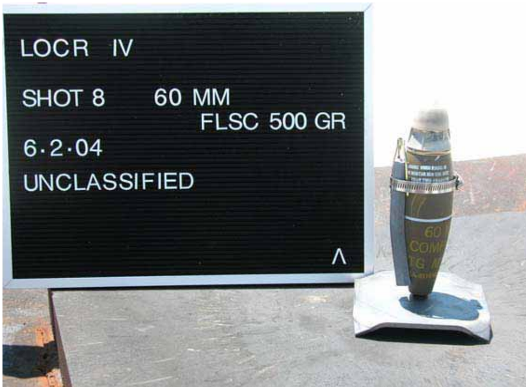
Figure 9-2. 60-mm mortar with FLSC strapped to the side.
