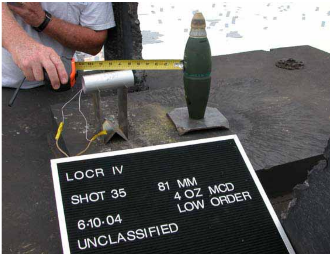
Figure 9-4. Positioning the MCD relative to an 81-mm mortar.
