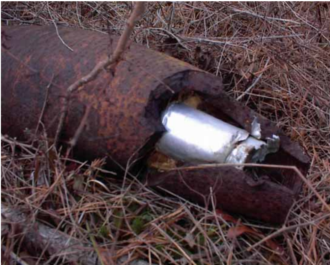
Figure 2-3. Cracked open 155-mm HE projectile with exposed Composition B behind aluminum booster charge.
