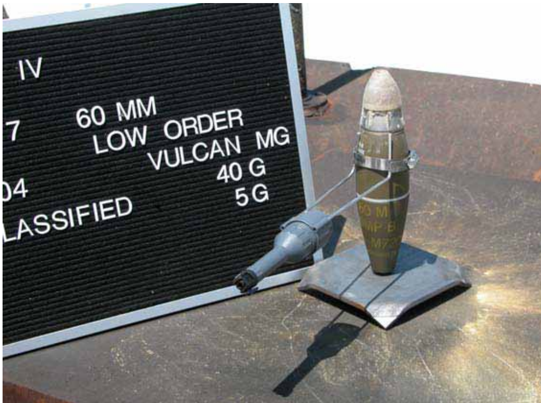
Figure 9-3. 60-mm mortar with Vulcan Shaped Charge. Standoff distance and elevation relative to the mortar were maintained by two wire legs secured to the mortar with a pipe clamp.
