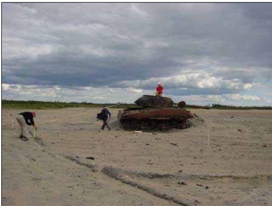
Figure 5-2. Establishing circular sampling pattern surrounding a tank target at live-fire bombing range impact area at Cold Lake Air Weapons Range.
