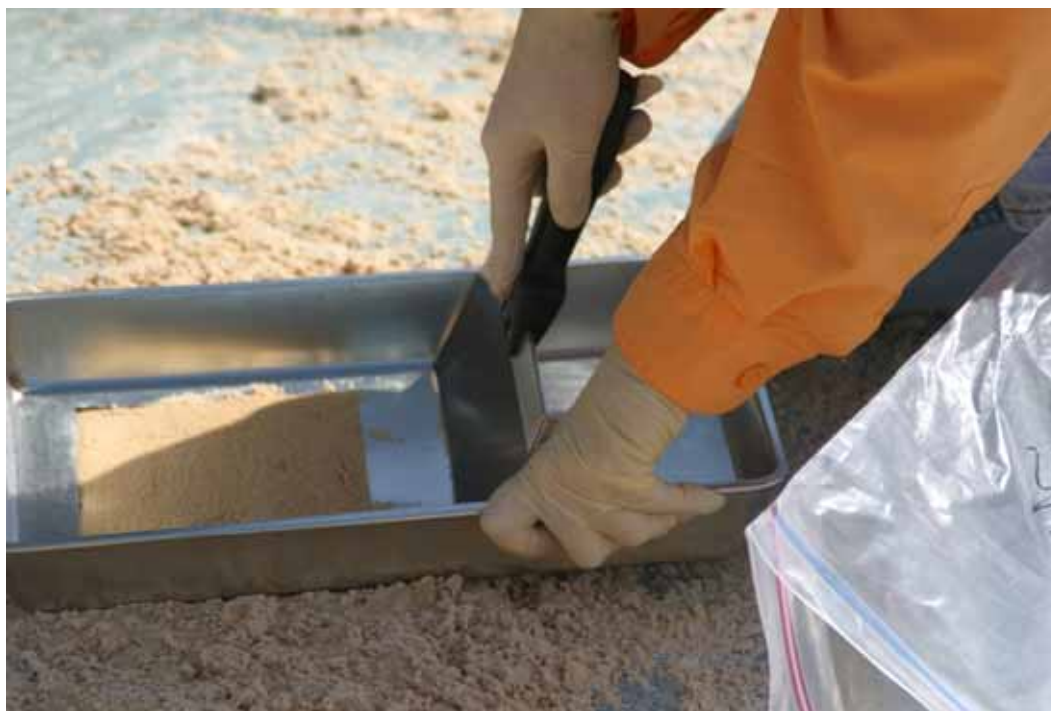
Figure 6-4. Surface sand sampling through a 10-cm \times 10-cm window cut into a 33-cm \times 23-cm baking pan.
