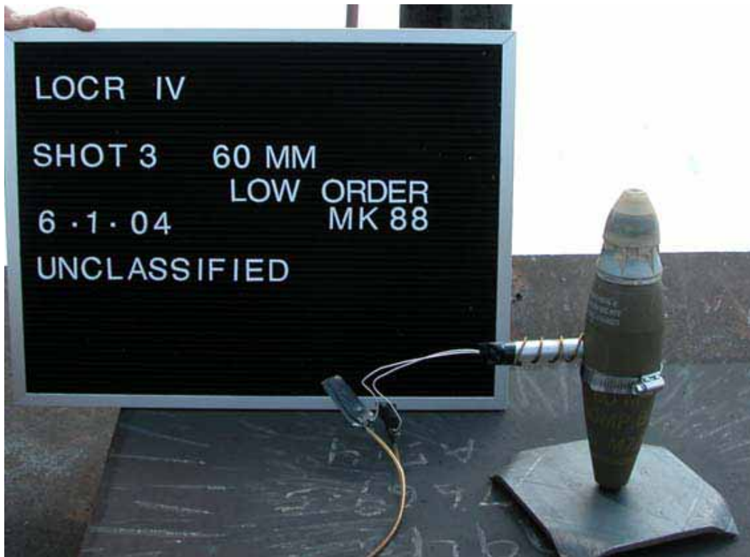
Figure 9-1. 60-mm mortar with MK 88 shaped charge held in place by a pipe clamp and coil of wire. Mortar rests on a metal plate to maintain upright orientation.
