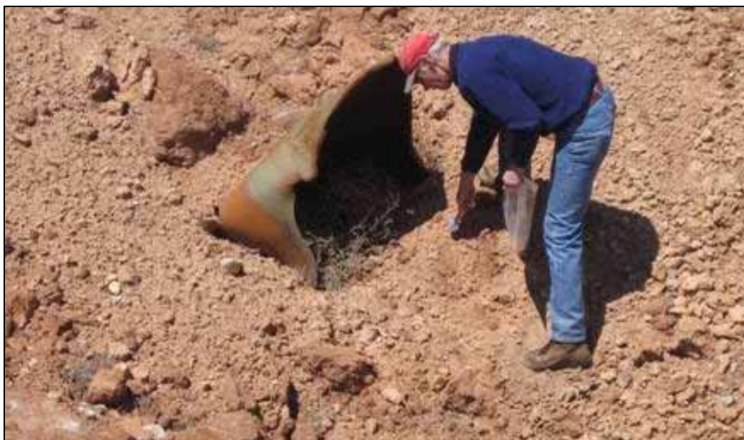
Figure 5-5. Sampling in front of low-order 2,000-lb bomb in crater at Holloman Air Force Base.
