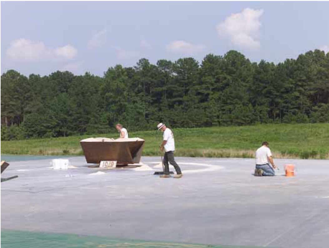
Figure 6-2. Field team recovers detonation residues by sweeping sand in concentric circles around detonation bucket.
