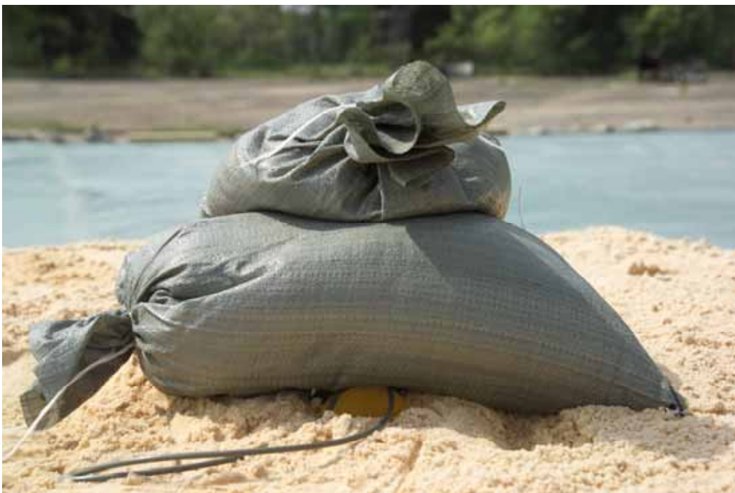
Figure 6-5. (a) 105-mm artillery projectile with Kinepak donor; (b) donor and projectile covered by two sand bags to promote high-order detonation by confining the donor.
