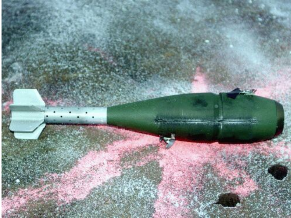
Figure 7-4. Effect of a shaped charge, showing groove blasted into projectile casing (Trial #2)
