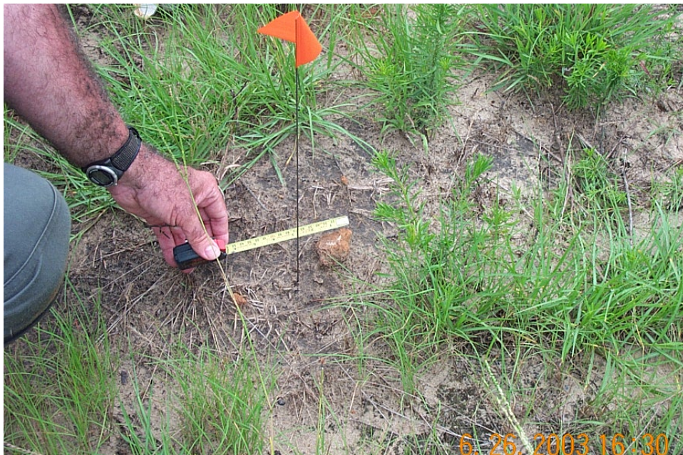
Figure 2-1. Chunks of Composition B from the partial detonation of an 81-mm mortar round found in the artillery impact area at Fort Polk, Louisiana.
