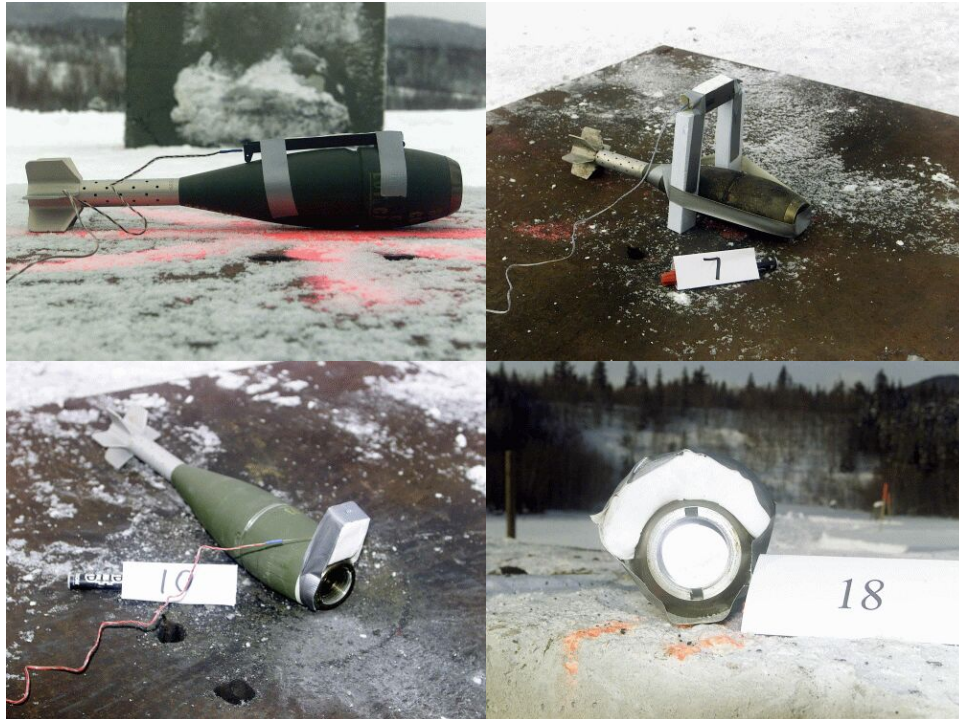
Figure 7-1. Configurations used in Method 1. Top left: small shaped charge longitudinal, minimal standoff. Top right: larger shaped charge, large standoff. Bottom left: Small block of C4 at the nose. Bottom right: Hemispherical configuration of C4 at the nose
