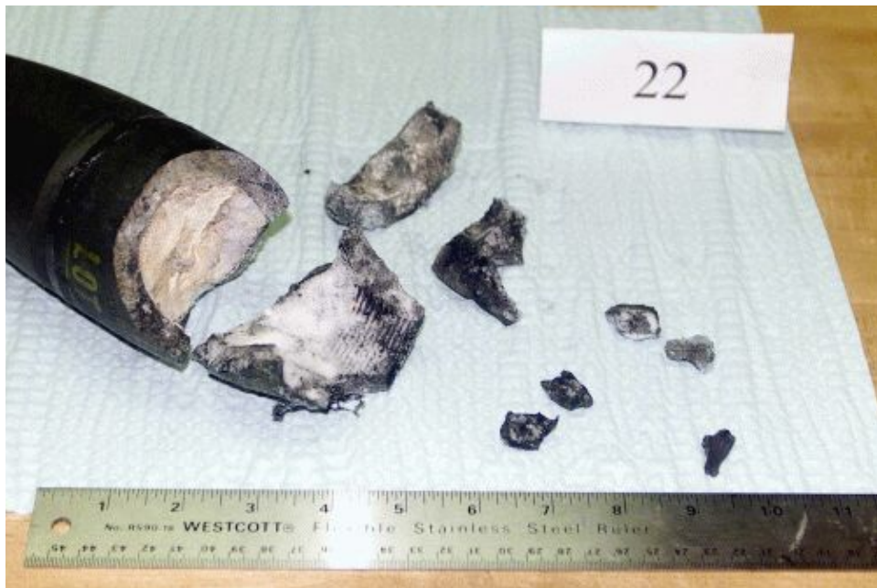
Figure 7-5. Cracked shell produced by C4 on the nose (Trial # 22)
