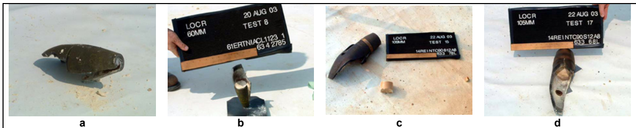
Figure 3-1. Typical low-order detonations. a. Casing and residual Composition B ejected from a 60-mm mortar, b. Casing and residual Composition B retained in a 60-mm mortar, c. Casing and residual TNT ejected from a 105-mm projectile, d. Casing and residual TNT retained in a 105-mm projectile
