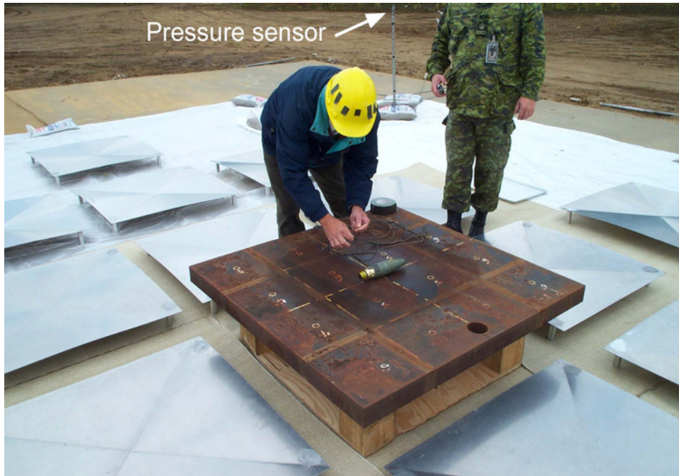
Figure 8-3. EOD staff install a detonator on a 60-mm mortar; location of the 5-m pressure sensor is shown at the back
