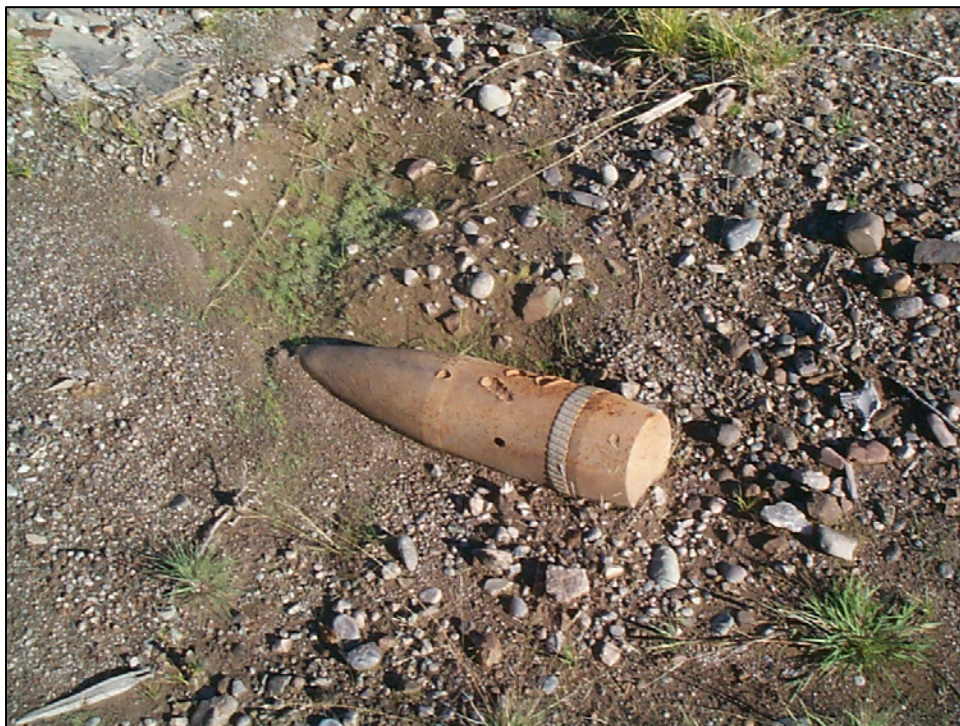
Figure 4-25. Hot spot sampled, Lawfield Impact Area, GPS location: 13973E 69357N, 155-mm artillery projectile
