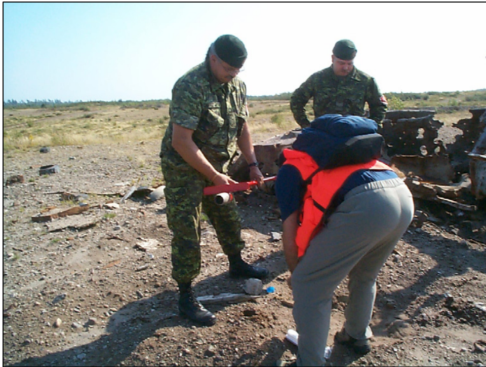
Figure 4-8. Core sampling with manual augers
