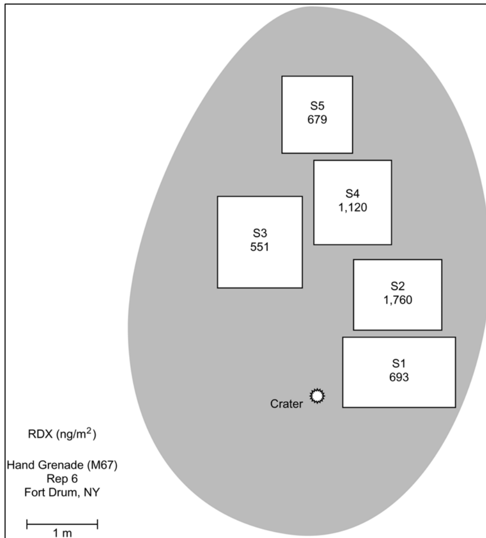
Figure 6-8. Residue plume #6 from live-fire detonation of M67 hand grenade with surface area sampled and concentrations of RDX determined
