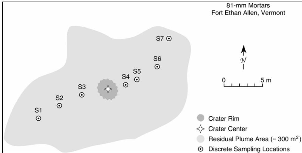
Figure 6-1. Residue plume from blowing in place an 81-mm mortar round with a block of C4, with sampling and crater locations marked
