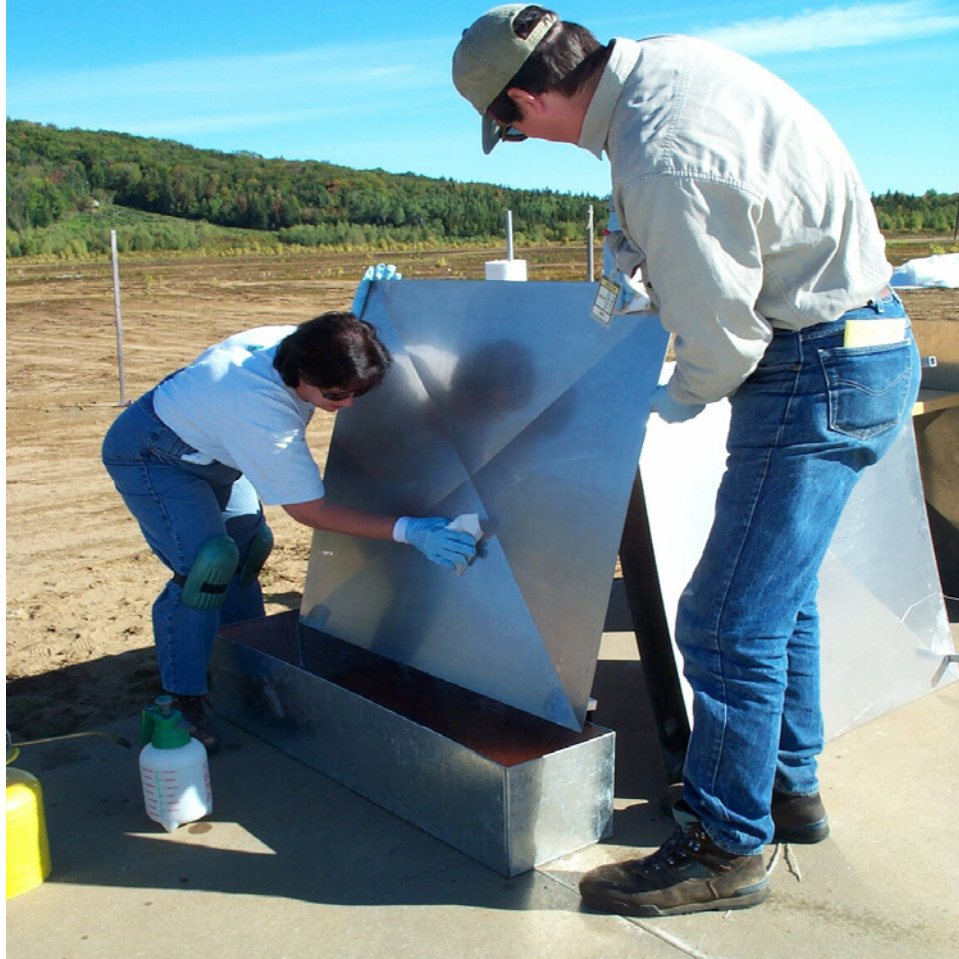
Figure 8-8. Washing of a witness plate after sampling
