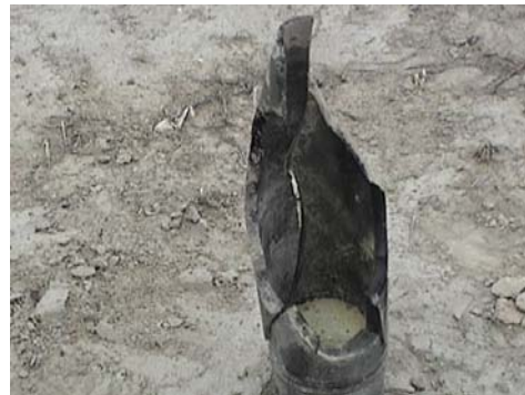
b. High explosive found in projectile casing after detonation
