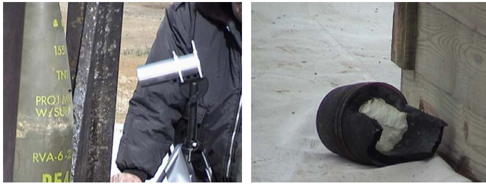
a. Predetonation setup of 155-mm projectile with MCD tool
