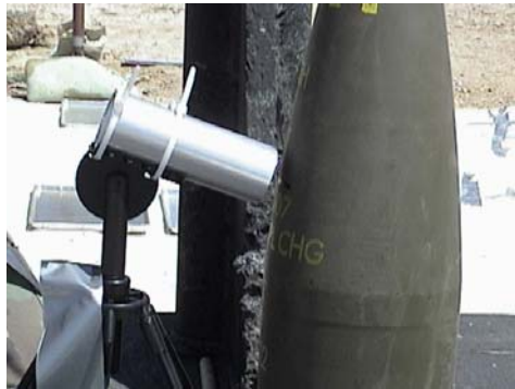
a. Predetonation setup of 155-mm projectile with MCD tool
