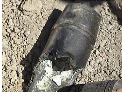
b. High explosive found in projectile casing after detonation
