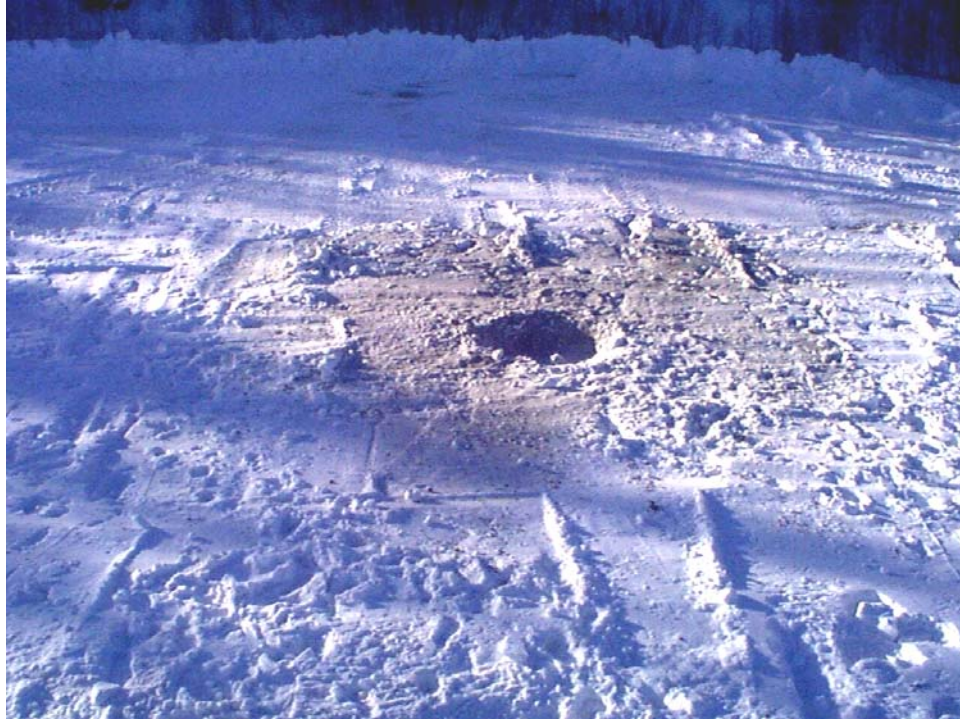
Figure 4-7. Soot plume of 60-mm mortar (crater is 1.5 m in diameter for scale)
