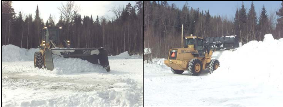
Figure 4-3. Front-end loader clearing the range after a trial
