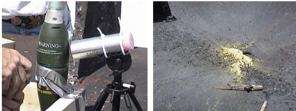
a. Predetonation setup of 81-mm mortar with MCD tool b. Large amount of high explosive found on table after detonation
