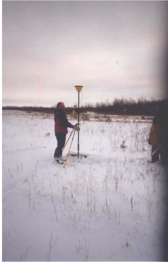
Figure 3-22. GPS location system for well land surveying
