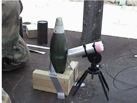
a. Predetonation setup of 81-mm mortar and MCD tool
