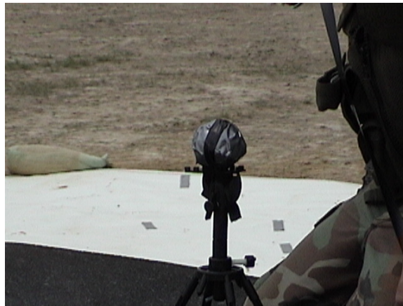
Figure 5-15. Tests 13 and 14, 6-oz C4 sphere for calibration
