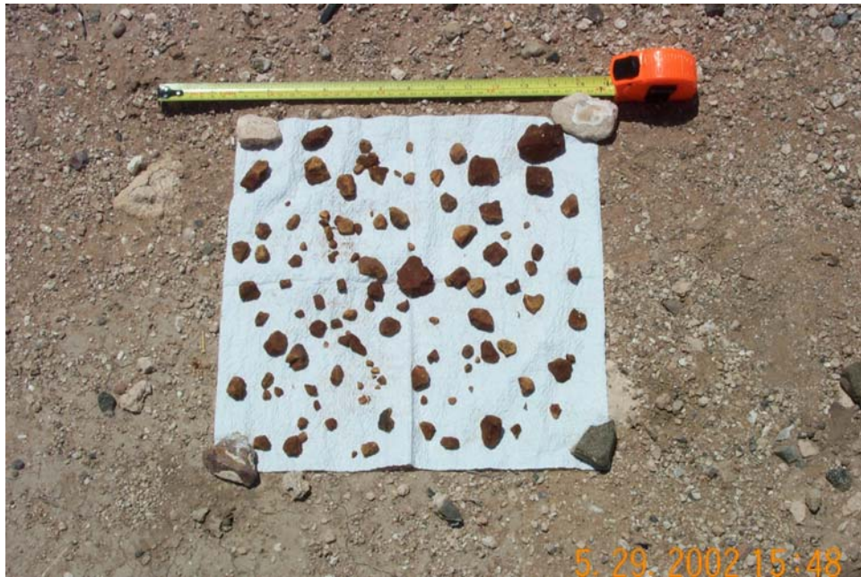
Figure 2-5. Photograph of pieces of TNT found within 10- x 10-m area sampled at Dona Ana Range, Fort Bliss, New Mexico
