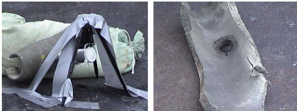
a. Setup of the MCD tool against 1/2-in. piece of fragment against sandbag
