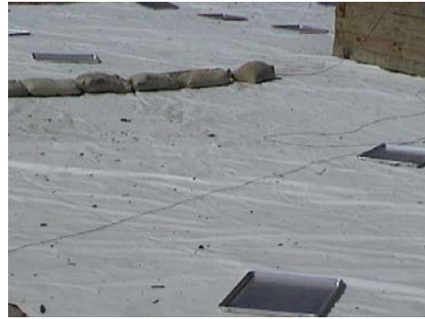
b. Postdetonation observation – Debris is charred wood
