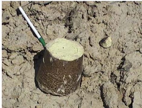
b. High explosive jettisoned from base of casing
