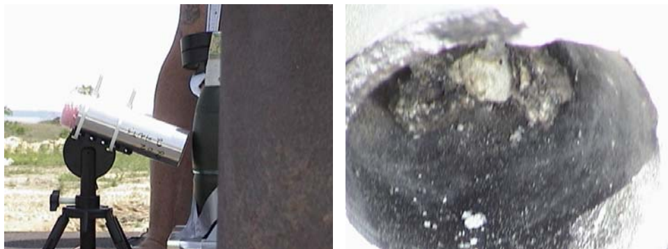
a. Predetonation setup of 81-mm mortar with MCD tool b. High explosive found in mortar casing after detonation
