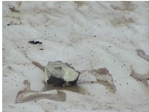
c. Chunk of TNT found on tarp after detonation
