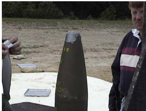
a. Predetonation setup of 155-mm projectile with C4 in fuze well
