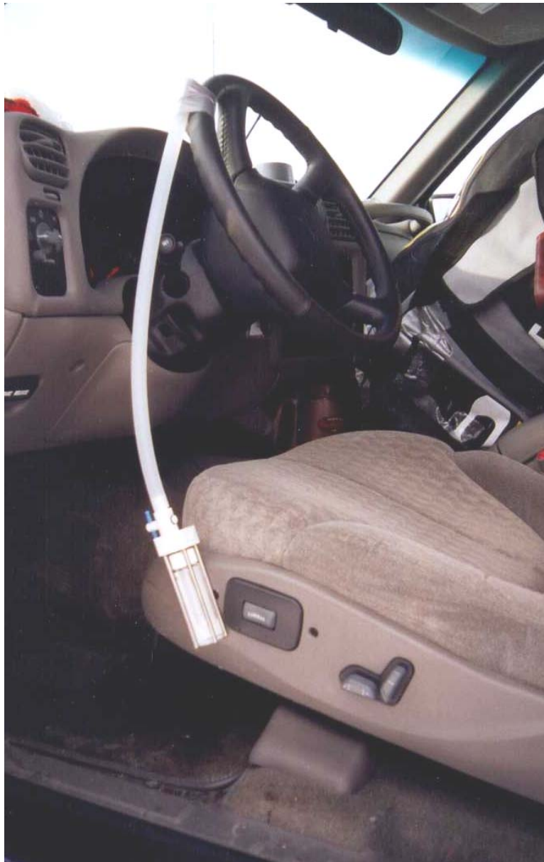
Figure 3-24. Double-needle device for sampling VOC's
