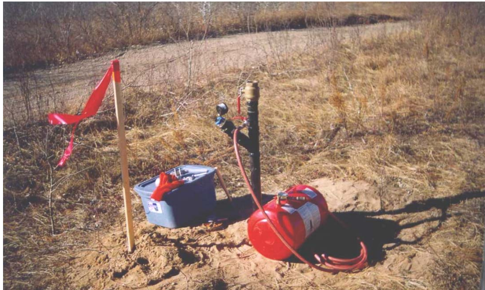
Figure 3-21. Device for injecting compressed air into well (slug tests)
