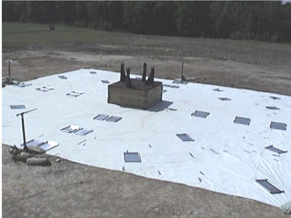
Figure 5-1. Setup of the system with witness plates, tarp, and pressure gauges
