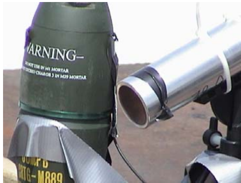
a. Predetonation setup against 81-mm mortar
