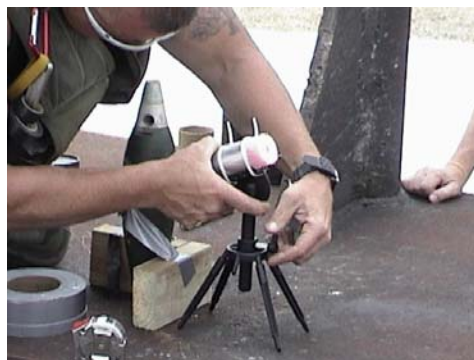
a. Predetonation setup against 81-mm mortar
