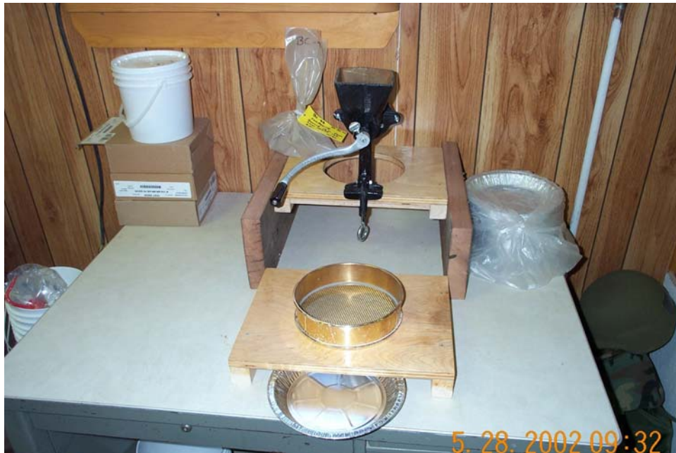
Figure 2-11. Photograph of manual soil grinder and sieves tested at Fort Bliss, New Mexico
