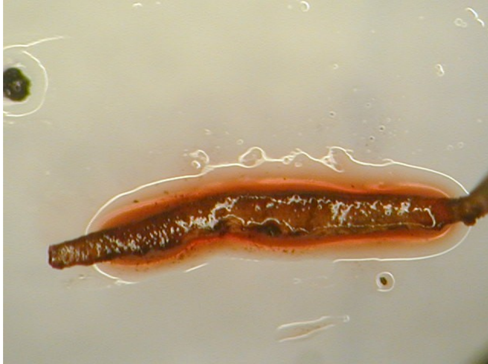
Figure 1-1. Development of red coloration in a fibrous particle of nitrocellulose when treated with a reagent that reacts with 2,4DNT. Particle was recovered near a firing point at Fort Richardson, Alaska
