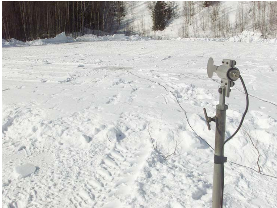
Figure 4-9. Pressure sensor 10 m from detonation site (in background)
