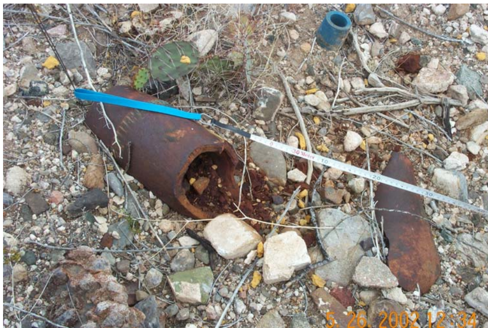
Figure 2-6. Photograph of low-order 155-mm round with chunks of TNT visible
