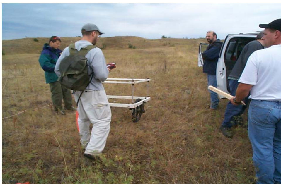
Figure 3-6. Well location proofing using EM-61
