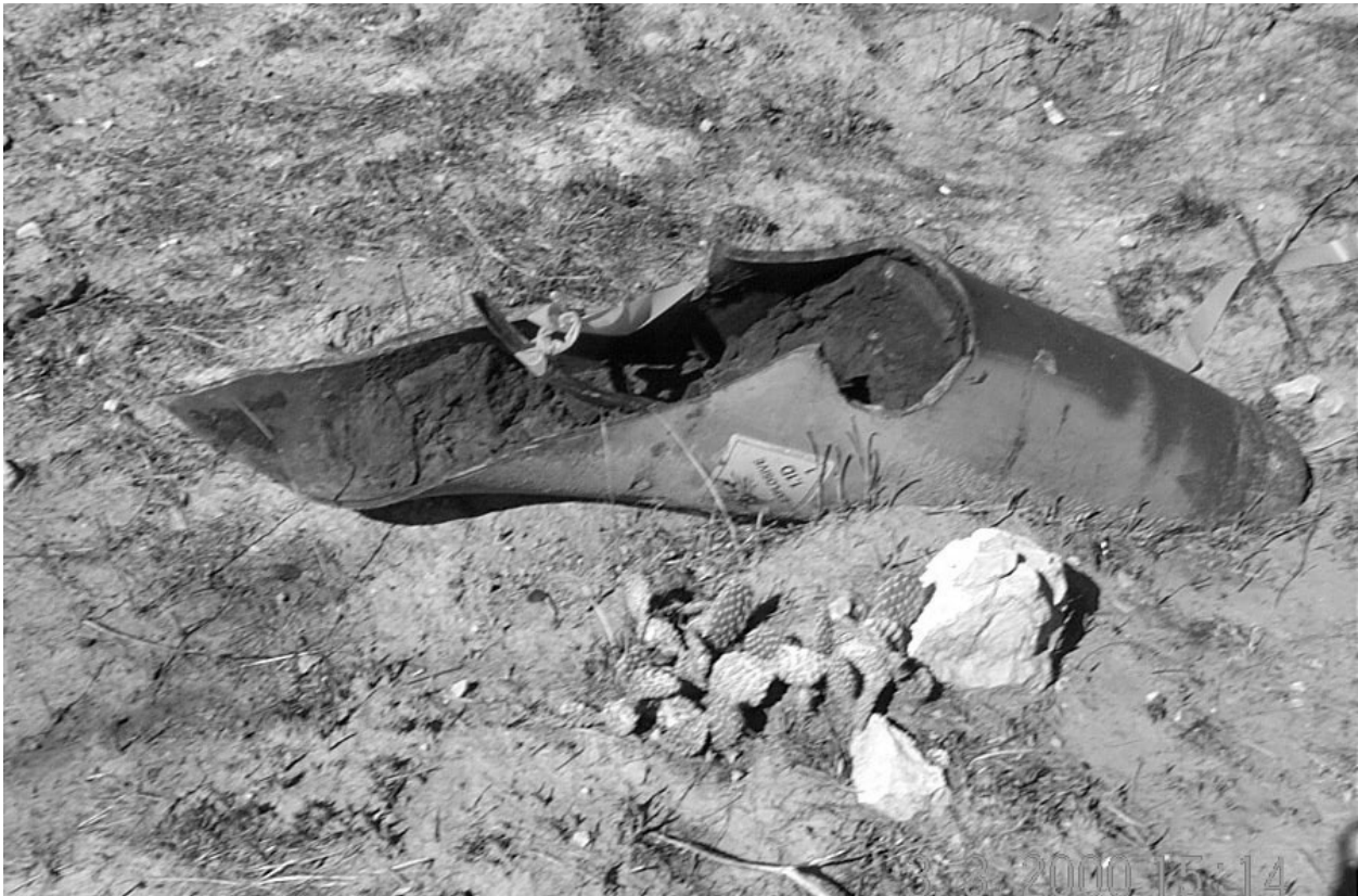
Figure 18. A 500-lb bomb that had undergone a low-order detonation, Central Impact Area, Camp Guernsey
