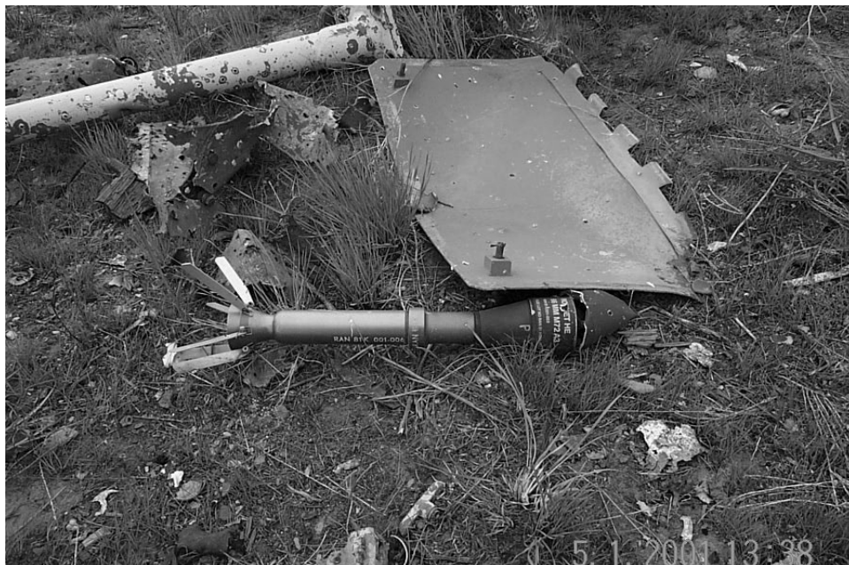
Figure 4. Ruptured LAW Rocket at Yakima Antitank Range
