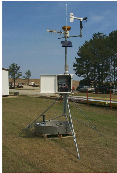
Figure 1. Automated weather station at Natural Resources Office
