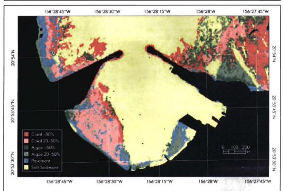
FIGURE 2. Georeferenced benthic habitat map of Kahului Harbor showing regions where coral or benthic algal cover are greater than 50% or between 20% and 50%. Soft sediment is defined as either sand or mud. Map was created using multispectral images from Ikonos satellite image shown in Figure 1 acquired on April 9, 2002. See Table 1 for area coverage of each component of habitat classification.
