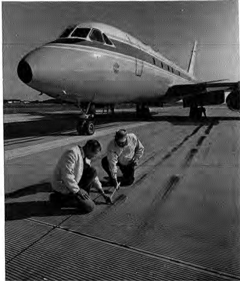
During May: Project engineer W. B. Horne, with T. J. Yager, examines effects of Con-Quair 990 landing on grooved runway at Wallops Station. Grooves—one inch apart, one-fourth inch wide, and one-fourth inch deep—increased friction on wet runways.
