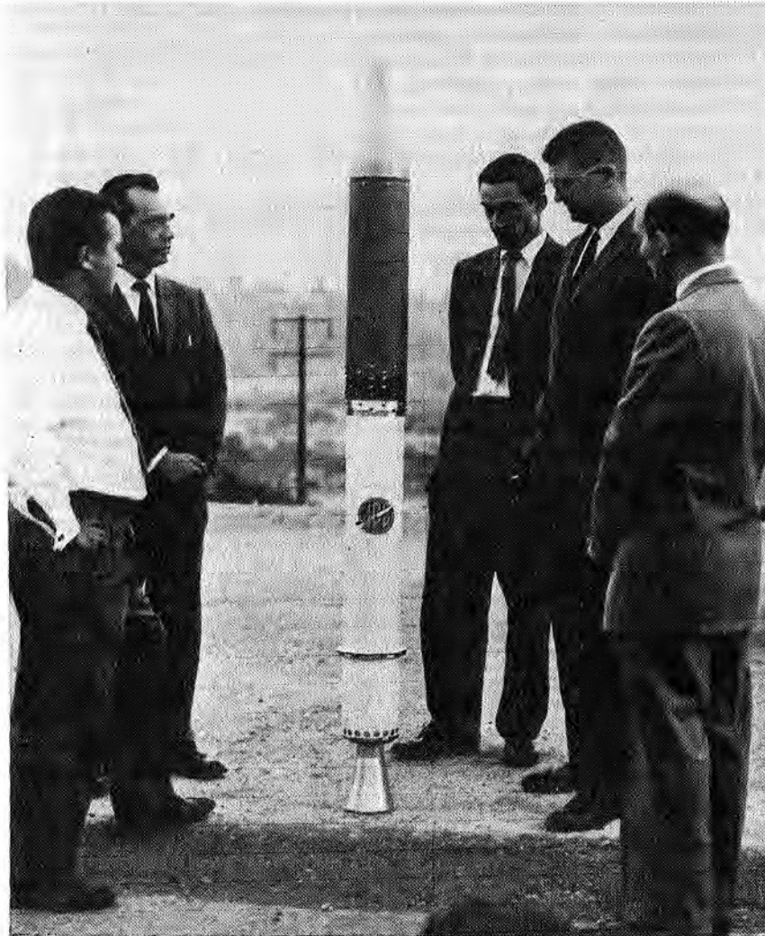
January 31: Tenth anniversary of first U.S. satellite, Explorer I, shown in 1958 photo with JPL scientists before ABMA-JPL launch. Still in orbit, 30.8-lb 80-inch assembly of instrumented upper section and final-stage solid-propellant rocket had traveled 1½ billion miles. Left to right are John Small; the late Dr. J. E. Froelich, JPL project director; Dr. Albert R. Hibbs; Karl W. Linnes; and Robert Victor. (U.S. Army photo)
