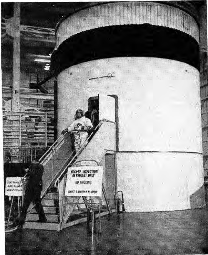
January 30: Engineering mockup of Saturn I orbital workshop readied for crew station review at Marshall Space Flight Center. Space-suited astronaut leaves full-size model of Saturn S-IVB rocket stage which will contain individual sleeping rooms, kitchen-dining area, laboratory work spaces, and waste-management area.
