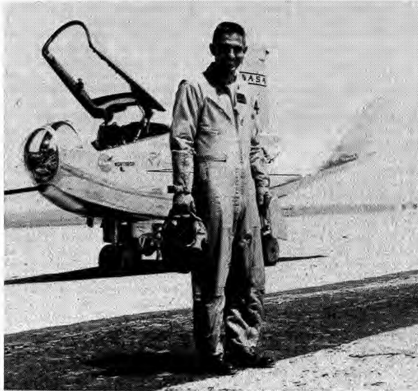
November 13: John A. Manke, NASA research pilot at FRC, stands before wingless HL-10 lifting-body vehicle which he flew in first powered flight, after air launch from B-52 aircraft. Manke reached 610 mph in NASA-USAF program to evaluate possible forerunners of reusable spacecraft. Eventual 1,000-mph speed was expected.
