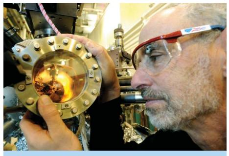
Argonne chemist Richard Rosenberg examines source material for an experiment to induce chirality into pre-biological systems at the Advanced Photon Source. Rosenberg used X-ray photoelectron spectroscopy to measure the secondary electron induced photolysis reaction rate of a model chiral compound adsorbed on a magnetic substrate. He found that changing the magnetization direction in relation to the high-intensity X-ray beam created an excess of one chirality over another.
