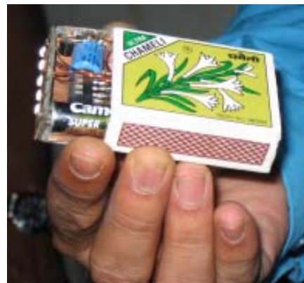
This matchbox flashlight was built at a Fab Lab in India. The LED-based device is powered by a single AA battery.
