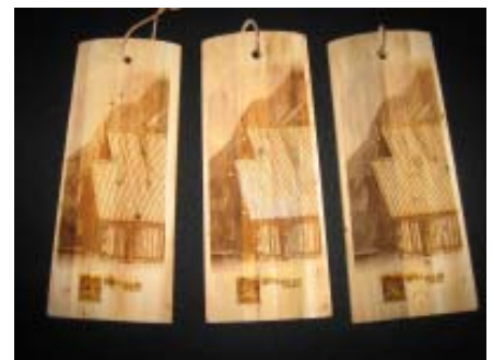
These etchings come from the Fab Lab in Tromsø, Norway, located above the Arctic Circle. The designs are designed on a computer and then “printed” onto the wood by extremely precise saws and cutters. One program can produce an unlimited number of replicas.
