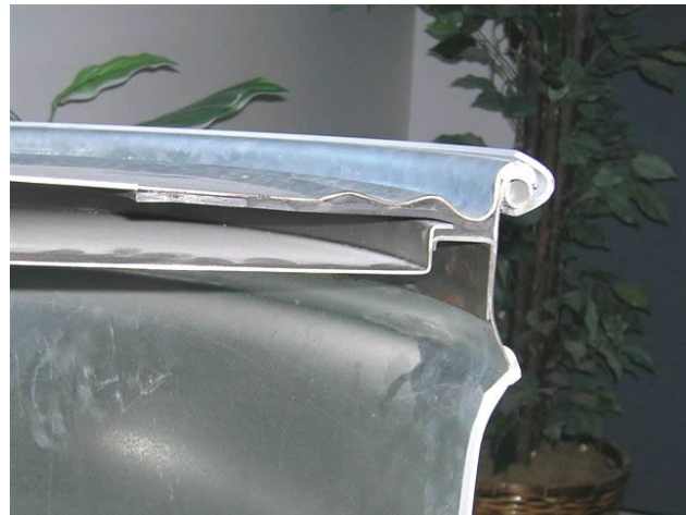
Exhibit 4-4: Cutaway of the Drum, Inner Lid, Outer Lid, Ring and Gaskets.
