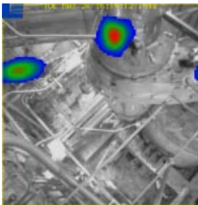
Exhibit 4-1: "Gammacam" Pictures Showing Areas of High Dose Rate.
